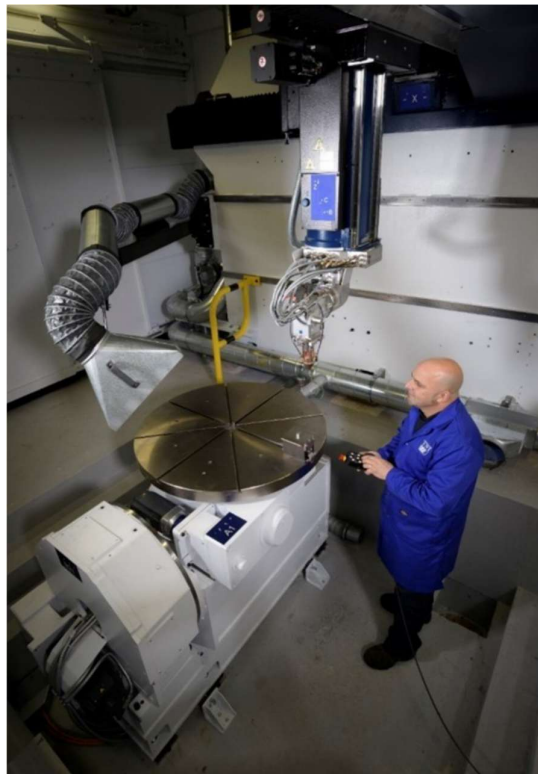
Figure 2 Laser DED Trumpf 7040 Equipment Inside
